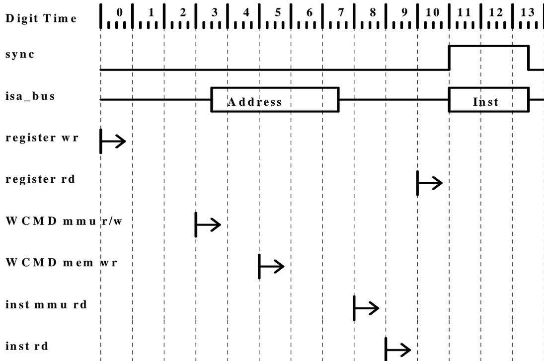
Memory accesses are always four clock cycles (of the input clock) in length. When not performing a memory access, the memory control signals are all inactive, the memory address is driven with all zeros, and the memory data bus is also driven with all zeros. The timing for a memory read is shown in the figure below.
