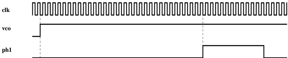
Even though the NEWT processor has begun operation at this point, the remainder of the system requires the **pwo** signal to be asserted to synchronize all system components to the NEWT machine cycle. These other components in the system require that the **pwo** signal change state at a specific time in the machine cycle, shown below.
