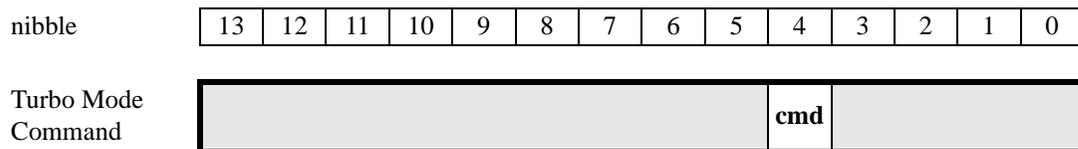
The options available for the Turbo mode are shown below. Turbo mode operates by “swallowing” clock pulses in the interface between the 18MHz clock input and the processor core. Even though clock pulses are swallowed, the external bus of the NEWT design always operates at the normal 360KHz speed.
