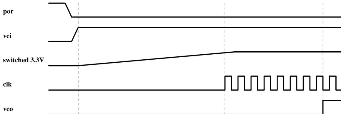
Once the **vco** signal is asserted, the NEWT exits the reset state and begins operation. It takes thirty-two clock cycles before the first **ph1** is output. At this point the NEWT is operating normally, at 1x speed.
