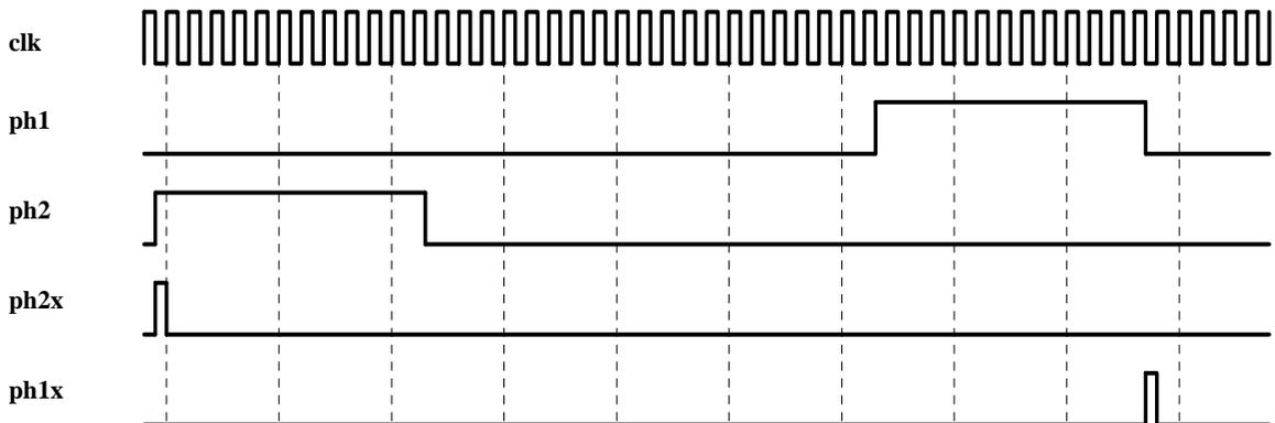
The ph1x and ph2x signals are used by the external bus portion of the design. A separate clock, called ph2c, is used by the logic of the CPU. When running in 1x mode ph2x and ph2c have the same timing. The details of this timing is shown in the figure below.
