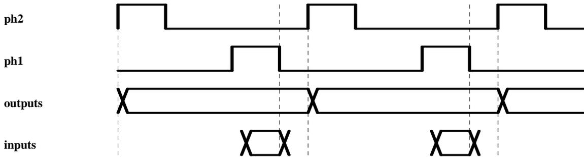
The NEWT CPU starts memory accesses of the physical memory at specific times during machine cycles, independent of the Turbo mode. Register accesses consist of four successive accesses. Note that register instructions are always executed in 1x mode, so all four physical memory accesses complete well before the end of the first bit time.
