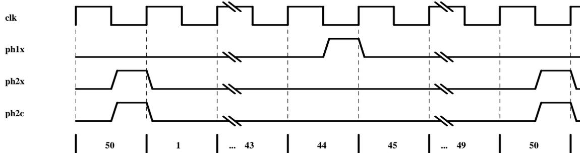
When running in one of the turbo modes, the external bus and ph2x are unaffected. However, the ph2c signal frequency is increased as shown in the figure below. Note that the ph2c signal is symmetric in all cases except for the 20x case.
