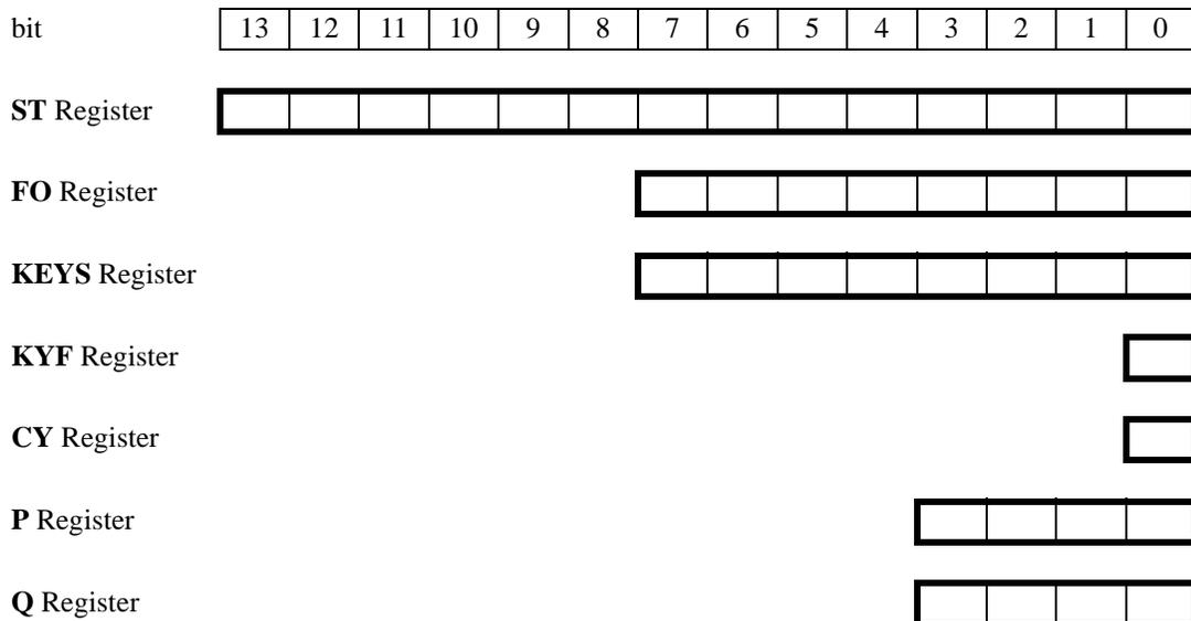
The P and Q registers are four-bit registers used to point to specific digits or ranges of digits in the general-purpose registers. When pointing to a specific digit only one of the registers is active at a time, but both are used when selecting a range of digits.
