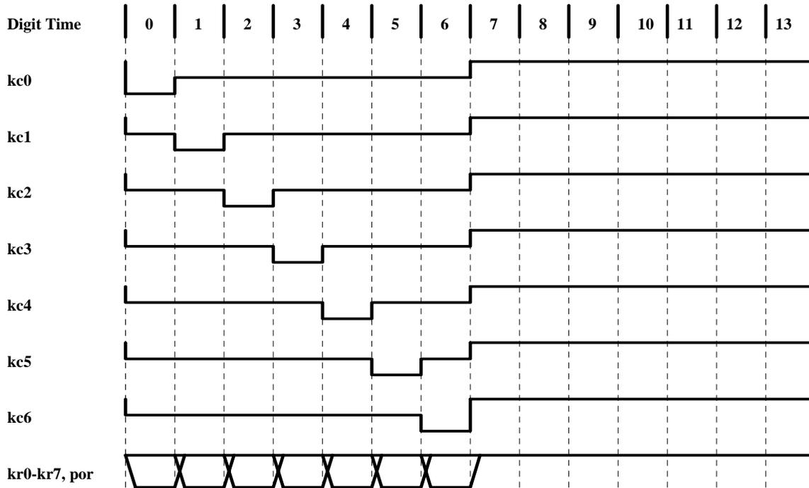
All Nut-compatible NEWT outputs change state relative to the rising edge of the **ph2** signal and all Nut-compatible inputs are sampled by the falling edge of the **ph1** signal. The original Nut documentation is vague on these timing details, but this is what can be inferred from the available information. This timing is shown in the figure below.
