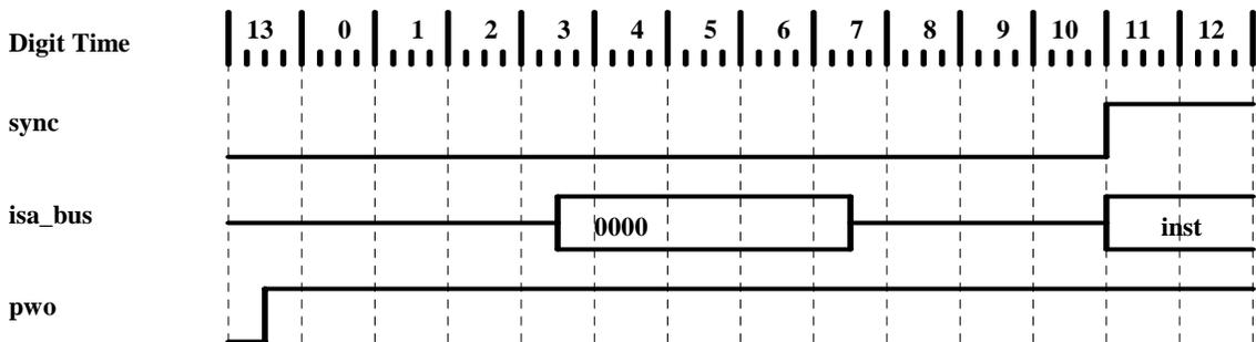
The **pwo** signal has unique timing, changing state between the **ph2** and **ph1** signal. The specific timing is shown in the figure below.
