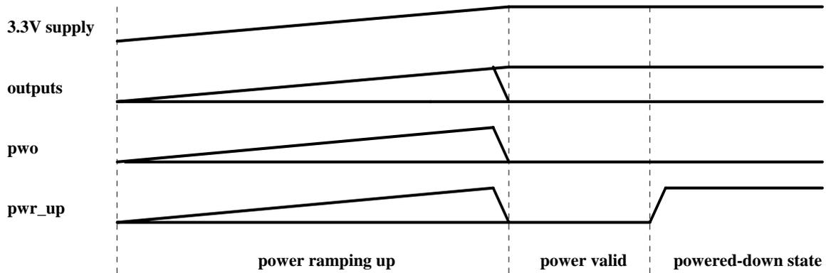
In the powered-down state the logic in the powered section watches for one of two conditions to initiate the power-up sequence. The first condition is a Low on the **por** input. This corresponds to a user pressing the ON key on the calculator. This condition is possible because the keyboard column output **kc0** is forced Low during power-down, while all of the keyboard row inputs have passive pull-ups.
