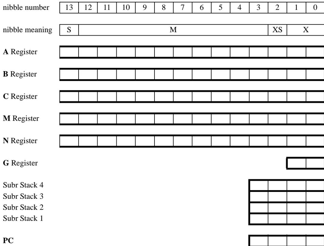
Normally both the exponent and mantissa hold 10's-complement BCD numbers. However, the CPU can also be operated in Hexadecimal mode, where the full binary encoding is allowed in the registers, for binary data or alphanumeric data. In the Hexadecimal mode all arithmetic operations operate in binary fashion, with binary carries from bit-to-bit and
