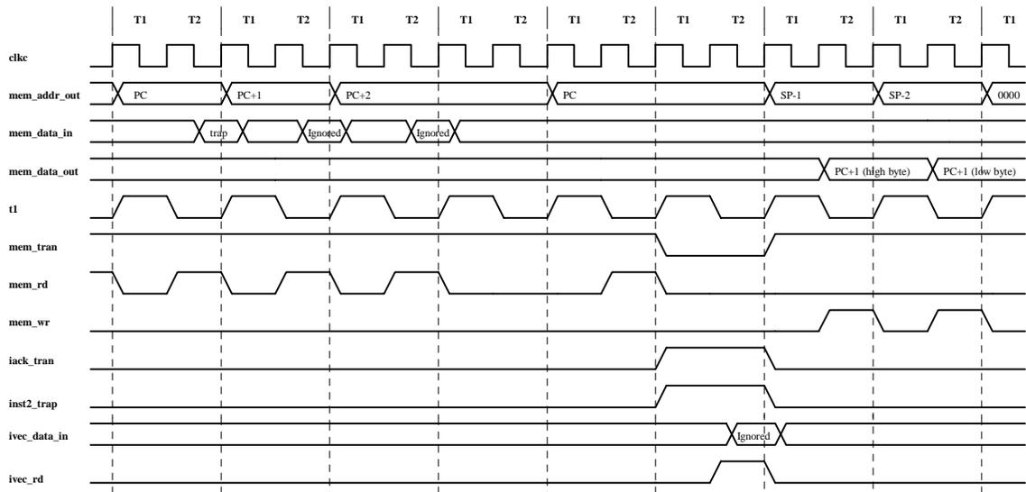
In the case of the Y90 CPU the **inst2\_trap** information should be latched outside the CPU to distinguish this case from both the **inst3\_trap** case and the normal reset case. The start of the illegal instruction in this case is the stacked PC value minus one.
