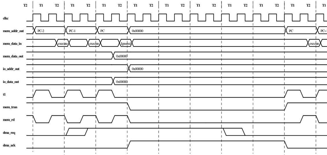
The DMA request controller in the Y90 MPU necessarily samples the **dma\_req\_bus** inputs, which changes the timing slightly. The diagram below illustrates this change. Also shown is the timing of the **dma\_ack\_bus** and the **dma\_prio\_out** signals. In particular, note that the leading edge of the **dma\_ack\_bus** signals are delayed by one clock cycle from the normal **dma\_ack** timing. The timing of the trailing edge of these signals is not affected.
