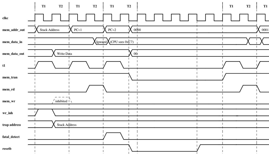
It is assumed here that the reset will clear whatever condition lead to signalling **wr\_inh** during a stack write. If this is not the case an infinite loop of traps can still result.
