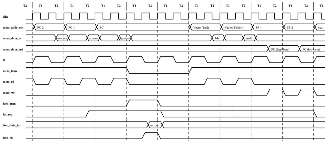
The interrupt controller in the Y90 MPU necessarily samples the **int\_req\_bus** inputs, and then goes into the edge-detect latch, which changes the timing slightly. The diagram below illustrates this change for Interrupt Mode 2. Also shown is the timing of the **int\_ack\_bus** and the **int\_prio\_out** signals.
