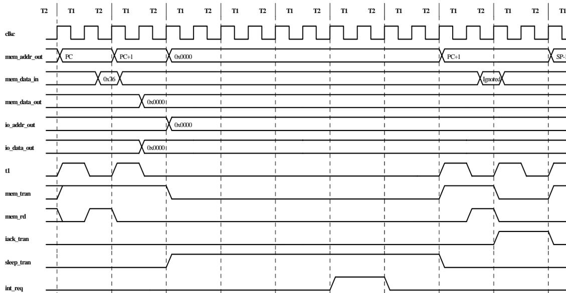
In the case where the Sleep state exit is caused by a maskable interrupt while interrupts are disabled the processor merely resumes execution at the address of the instruction following the SLP instruction, without going through an interrupt service routine. Note that the minimum width of the **sleep\_tran** signal is two clock cycles.
