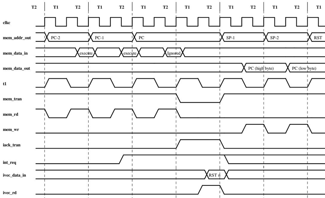
The use of an RST instruction is enforced by the hardware, which only uses bits 5-3 of the **ivec\_data\_in** bus to create one of the eight possible RST instructions.
