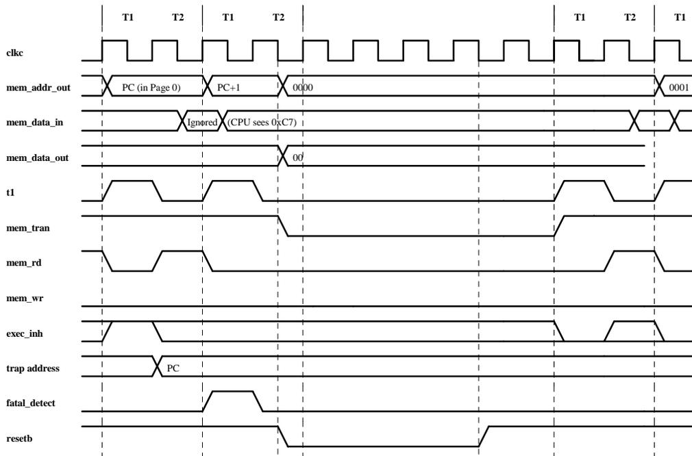
It is assumed here that the reset will clear whatever condition lead to signalling **exec\_inh** during a Page 0 access. If this is not the case an infinite loop of traps can still result.
