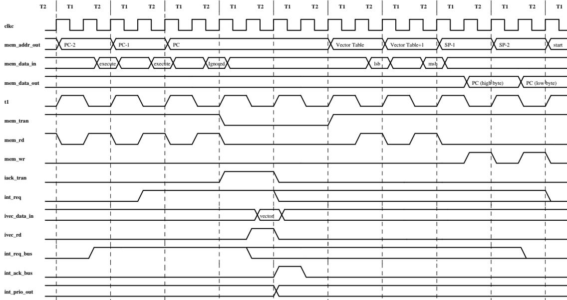
Although Interrupt Mode 2 is the preferred mode for use with the interrupt controller, the design allows the use of any interrupt mode. In Interrupt Mode 0 or 1 it will be necessary to use the **int\_ack\_bus** signals to externally latch the information about which interrupt is being acknowledged. This is because Interrupt Modes 0 and 1 will branch to a common interrupt service routine, rather than the individual routines possible in Interrupt Mode 2.
