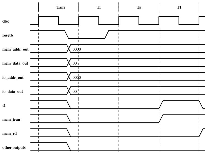
In the case of the Y90 MPU the **resetb** signal is an output, generated from the **reset\_bus** input signals or internal error conditions. The **reset\_bus** input signals are synchronized and filtered to generate the **resetb** signal synchronous with the falling edge of the **clk** signal.
