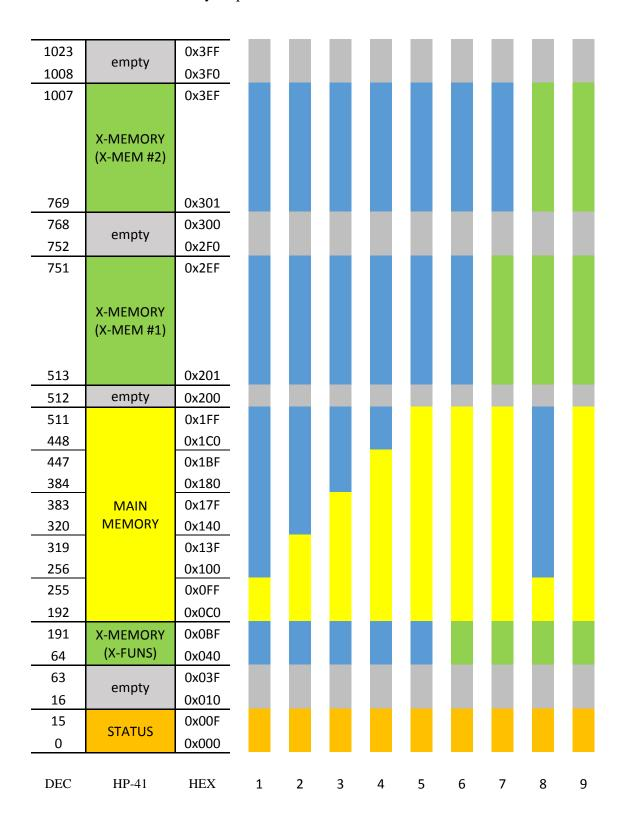
Even though the MAXX module automatically compensates for other memory modules present in the HP-41, it really only makes sense to use the MAXX module by itself to keep as many ports as possible free for other uses
