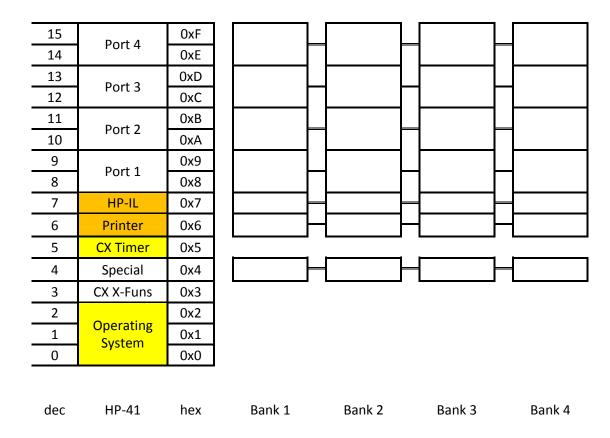
Not shown in the figure above is the special bank-switching employed by the HP-41CX. In the HP-41CX pages 3 and 5 share a bank-control bit (only banks 1 and 2 are present) to allow an expanded set of X-Functions. This bank-switching is completely independent of the bank-switching in the MAXX module.
