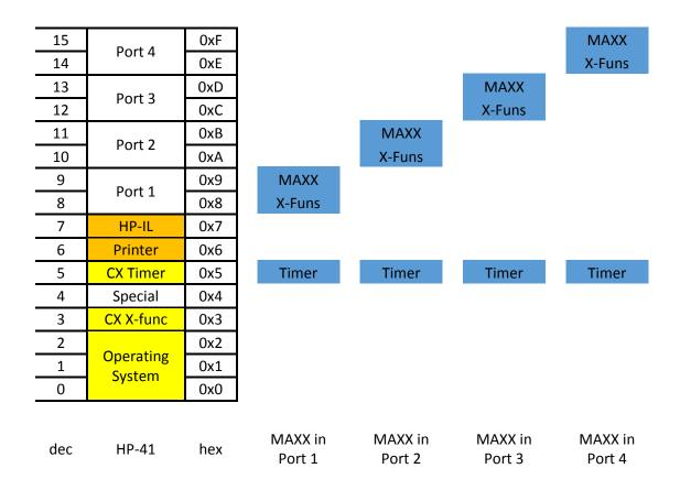
If the MAXX module is used in a 41CX the lower half of the Port where the module resides will be available for other uses, but the MAXX software always resides in the upper page of this Port.
